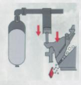
seals and protective wear sleeves make servicing the tramp iron relief system quick and easy. The lift on a Rollercone II enables it to pass objects up to  $5^{1/2}$  inches (140 mm).
